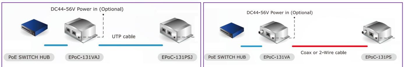
3. Verify that green Link LED of each device is ON, these devices had been previously joined in factory.
